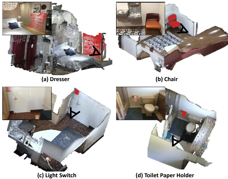
Figure 5: Qualitative results of open-vocabulary tasks. Our open-vocabulary instance segmentation is able to handle different queries. For each query, a corresponding 3D point cloud and a 2D image are provided. The segmented parts are marked in red.
